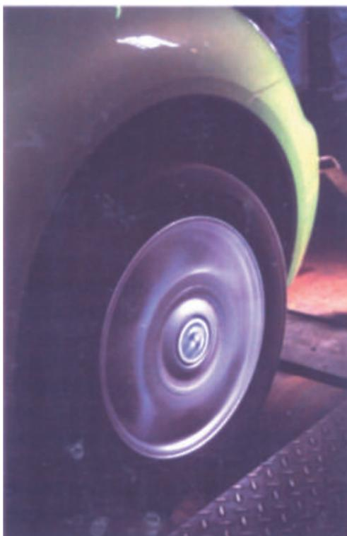
The rolling road measures power at the wheels and then records transmission losses on the overrun, before computing a figure for power at the flywheel.
